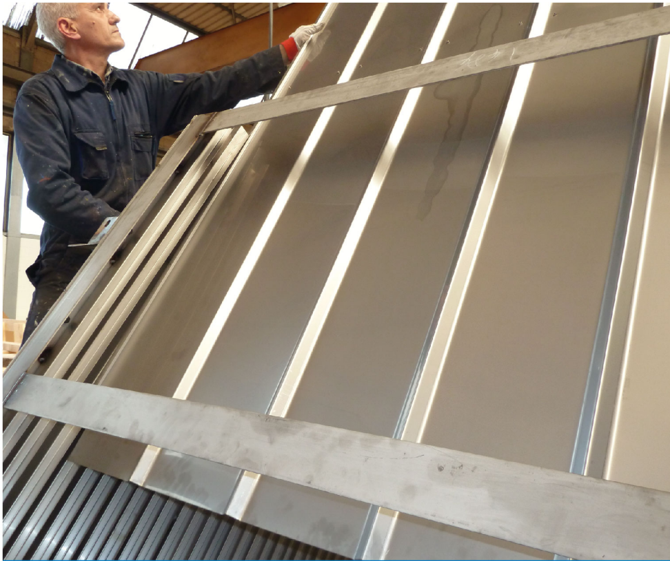
AISI-316L plate-type lamellae being assembled in module pack for placing in clarifier tank
