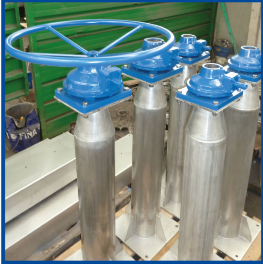
Operating pedestals, or headstocks, for manual and/or actuated service
